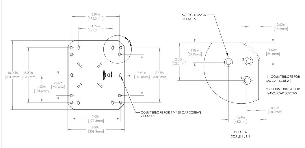
NOTE: CONFIGURATION FOR METRIC AND IMPERIAL TABLE MOUNTING IS THE SAME ON EACH OF THE FOUR CORNERS
