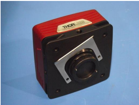
Figure 15 Loosening the C-mount and IR-Block Filter Assembly from Camera
