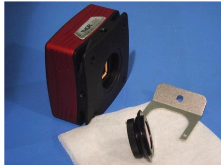
Figure 15 Loosening the C-mount and IR-Block Filter Assembly from Camera
