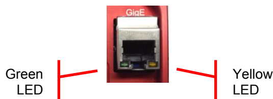
Figure 26 Detail of Gigabit Ethernet Port, showing the two status LEDs.
