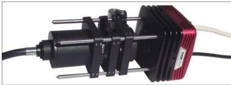
Figure 9 Camera Shown as Part of a 60 mm Thorlabs Cage System
