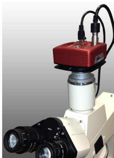
Figure 7 Camera Shown on Microscope Using C-Mount Adapter
