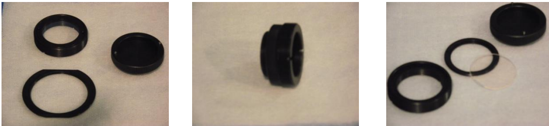
Figure 17 Removal of the IR-Blocking Filter from the Assembly
