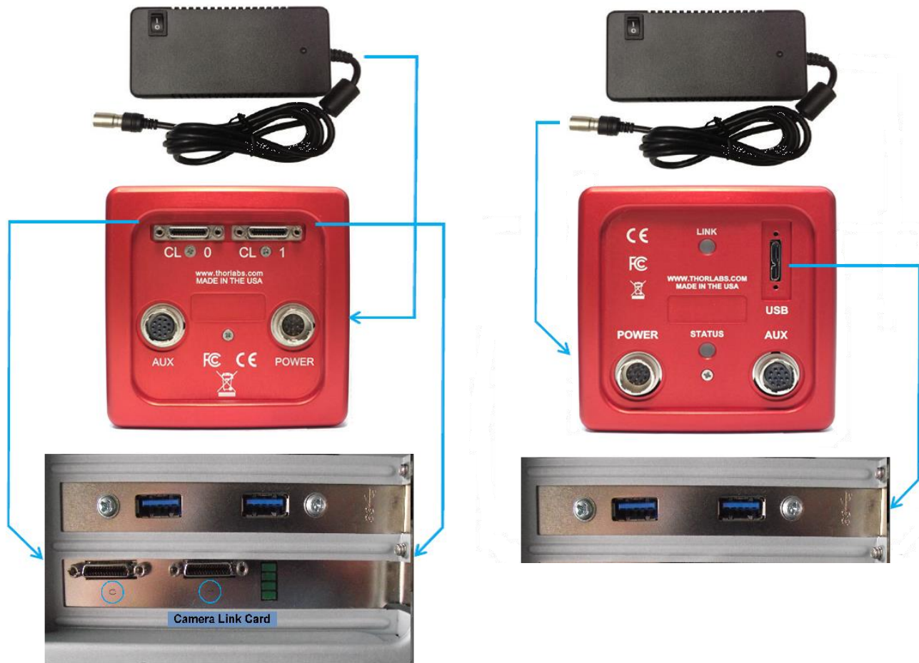
Figure 4 Diagram of Connectors on CL configuration (Left) and USB 3.0 (Right)
