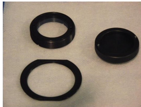
Figure 16 Removing the C-mount and IR-Block Filter Assembly from Camera Body
