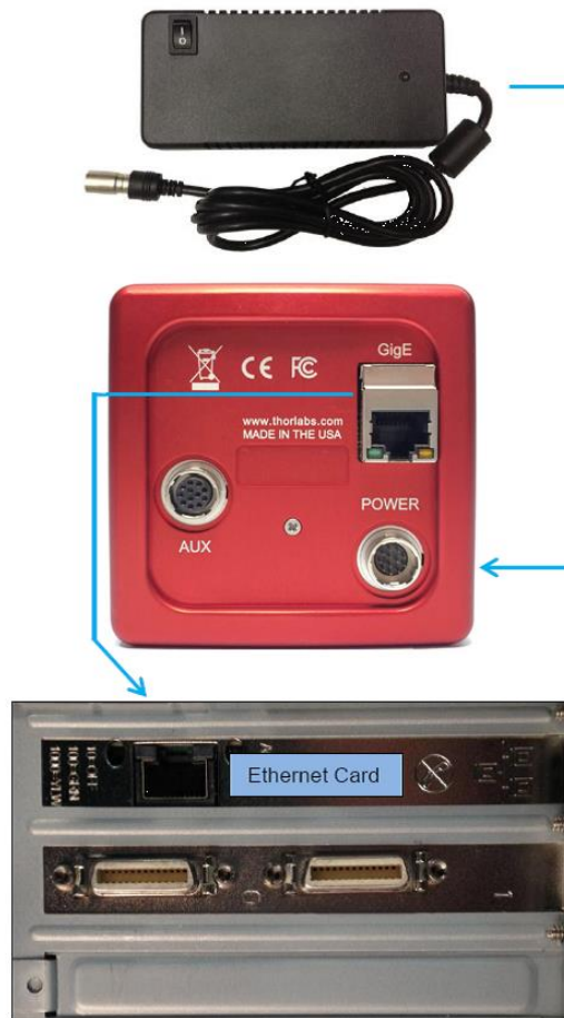
Figure 3 Diagram of Connectors on GigE configuration
