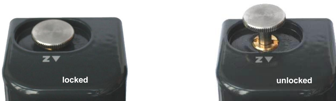
Figure 13 Reference Length Adjustment
