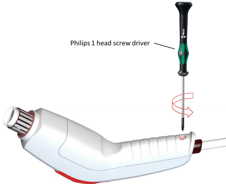
Figure 15 Remove Housing Fixation Screw
