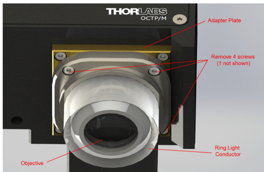
Figure 20 Removing the Objective
