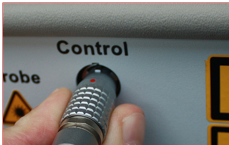
Figure 17 Installation of the Electrical Control Connector at the Base Unit
