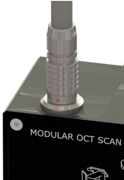
Figure 16 Installation of the Electrical Control Connector at the OCTP
