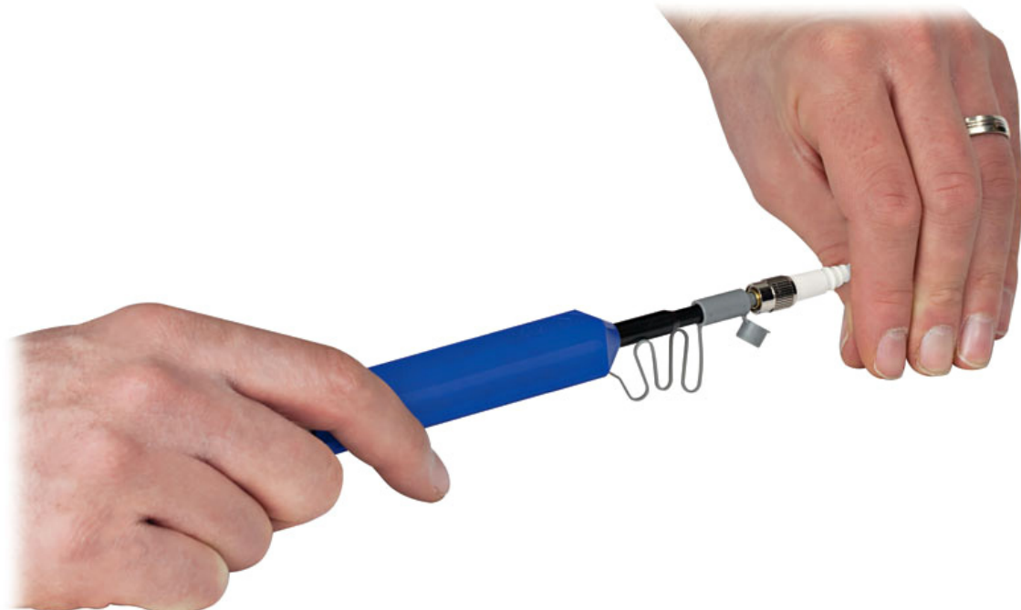
Figure 4 Cleaning Fiber Connectors
