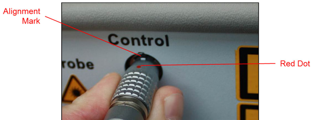
Figure 11 Installing the Electric Connection Cable at the Base Unit
