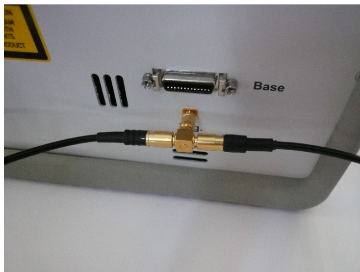
Figure 14 External Trigger Attached using an SMB Tee Connector
